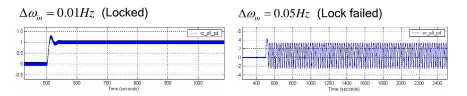
2.  $\zeta$  and loop bandwidth (1<sup>st</sup> pole) can not be independently determined.
