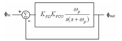
Closed loop gain (transfer function): 2<sup>nd</sup> order low-pass filter
