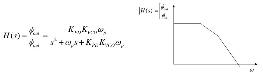
Note that input and output of PLL model are 'phase'.
