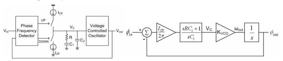
→ Ripple reduction with small  $C_2 (\approx C_1/10)$ → Simplification as 2<sup>nd</sup>-order system
